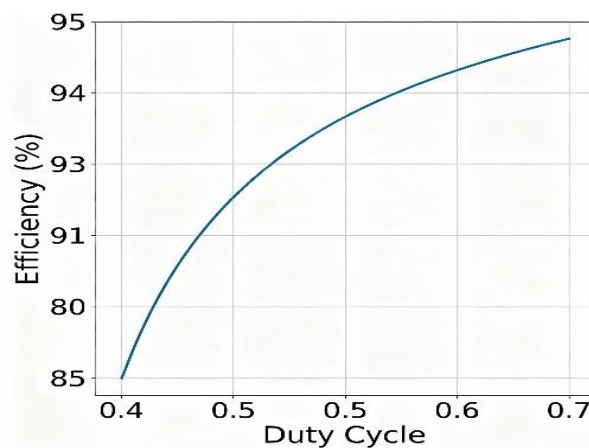
Figure 13: Curve shows duty cycle vs efficiency of DC-DC converter
